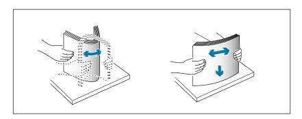
4. Place the paper into the paper input tray, **print side down**. You can insert **up to 150 sheets** of 20 lb plain paper.
